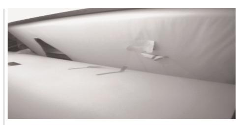
PAPER BREAKS: Camera monitoring can document paper faults and reel problems, making it easier for Norske Skog to solve such problems in cooperation with the customer.
